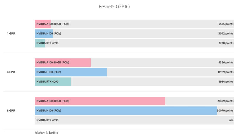
Figure 5.2.1. Comparison of GPU Performance: A100 vs. H100 vs. RTX 4090
